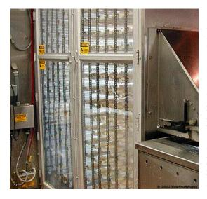
In order to heat the doughnuts to just the right temperature, the proof box machine has to keep the heat and humidity at very specific levels for a certain amount of time. If it gets too hot or humid, the machine opens up vents in the side of the proofer to let some air out. Krispy Kreme doesn't publicize the exact proofer settings, as they're part of the secret recipe. The dough spends 15 to 20 minutes in the proof box.
